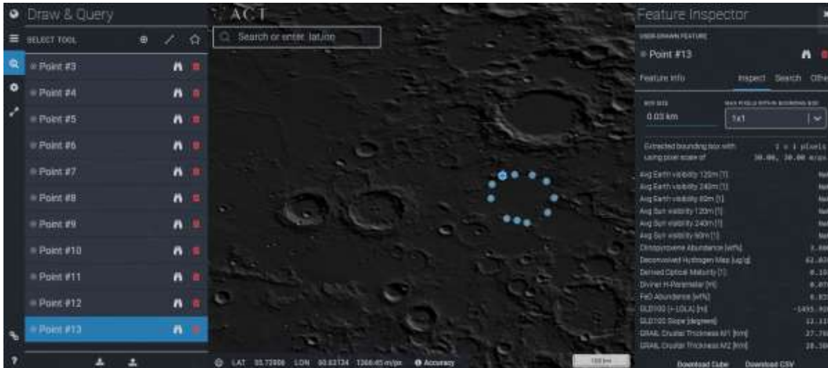
Figure 3. Using the “Draw and Query – Point Tool” to measure the rim of a buried or degraded crater.
