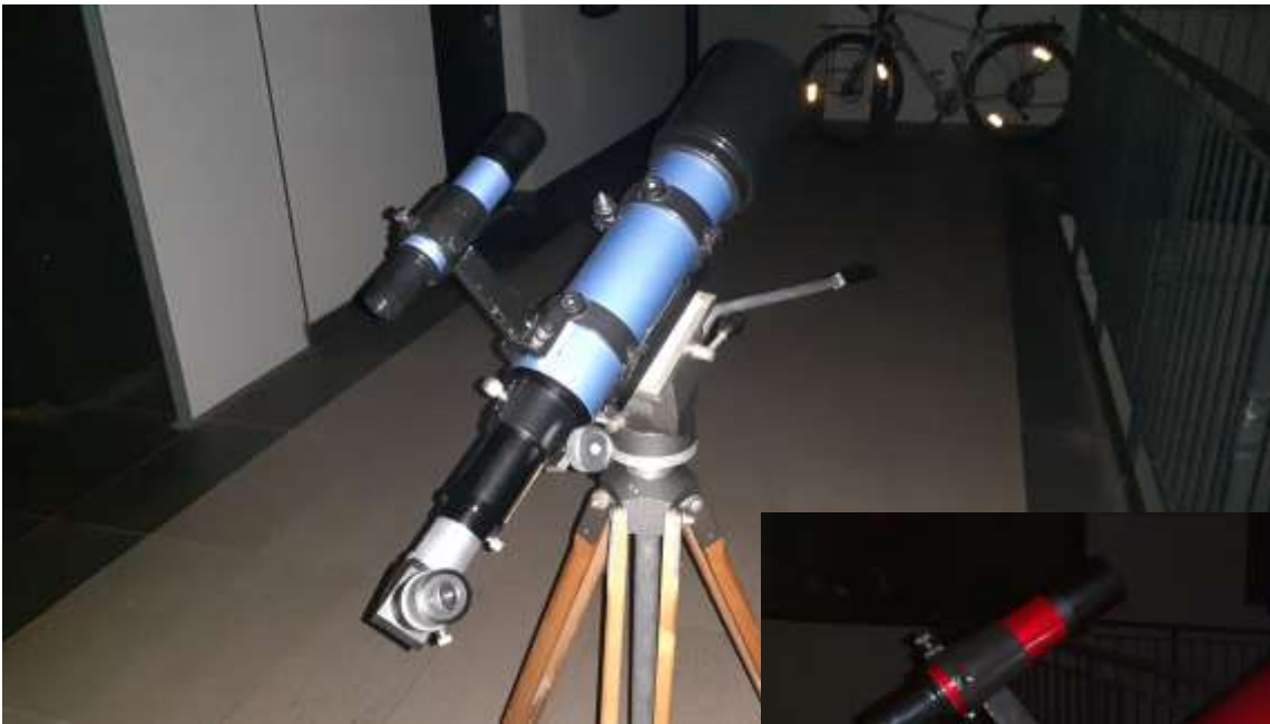
3 (left): 70/500mm ref. The original owner sold this to me for the price of a Plossl eyepiece.... I felt that I might have problems with chromatic aberration, but as it turned out, this problem is
