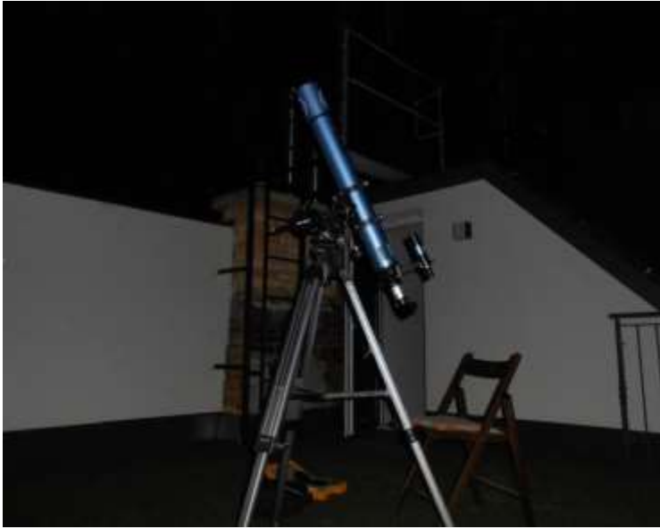
1 (left): 80/900mm refractor. I used it for open clusters in general and for observing the Moon.
