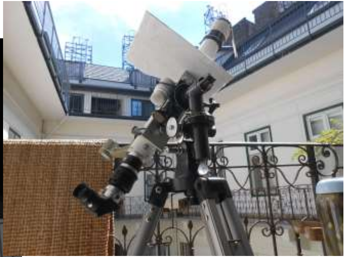
1 (left): 80/900mm refractor. I used it for open clusters in general and for observing the Moon.
